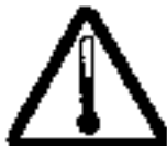
General hot surface warning
